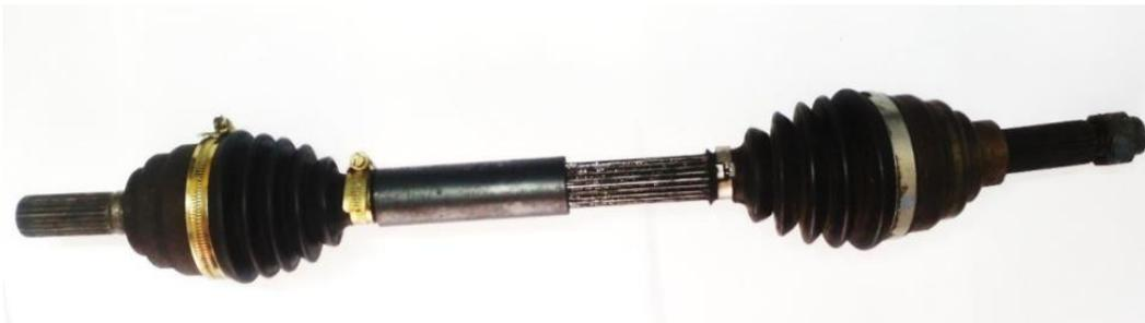
Developed telescopic shaft for all-terrain vehicle for providing constant velocity and in the process of filing patents.
